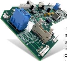
Through-hole technology (also spelled "thru-hole"), refers to the mounting scheme used for electronic components that involve the use of leads on the components that are inserted into holes drilled in printed circuit boards (PCB) and soldered to pads on the opposite side either by the manual assembly (hand placement) or by the use of automated insertion mount machines.
