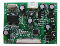
The mixed technology PCB assembly has the properties of both surface mount technology (SMT), and through-hole technology, hence the name. Thus, these assemblies are most commonly used in applications, which require the combination of both through-hole and SMT assemblies.
