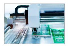
Surface Mount Assembly Using Machinery (pick and place machine) Use of led or through-hole parts has become rarer and is now discouraged by assemblers. It is far more efficient to machine assemble an electronic circuit if it is completely populated with surface-mounted components.
