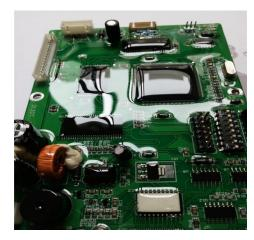
The conformal coating material is a thin polymeric film that conforms to the contours of a printed circuit board to protect the board's components. Typically applied at 25-250 µm thickness, it is applied to electronic circuitry to protect against moisture, dust, chemicals, and temperature extremes.
